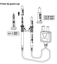
For CAT III or CAT IV environments, use the test leads with the probe tip guard cap fixed firmly. Without the probe tip guard cap, the test leads can be used in CAT II environment ONLY.
