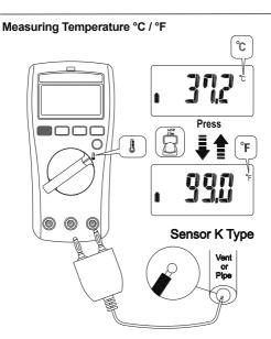
Dial the switch and press the Function button to select the measuring function. (°C / °F)
