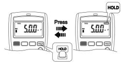
The meter will beep continuously and the display will flash if the measured signal is larger than the display reading by 50 counts. (However, it can not detect across the AC and DC Voltage / Current).
