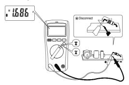
Dial the switch and press the Function button to select the measuring function.
