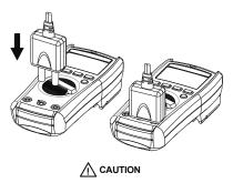
Make sure that test leads are firmly connected to the V-COM terminals of the correct instrument, and the instrument have to switch to PV mode.
