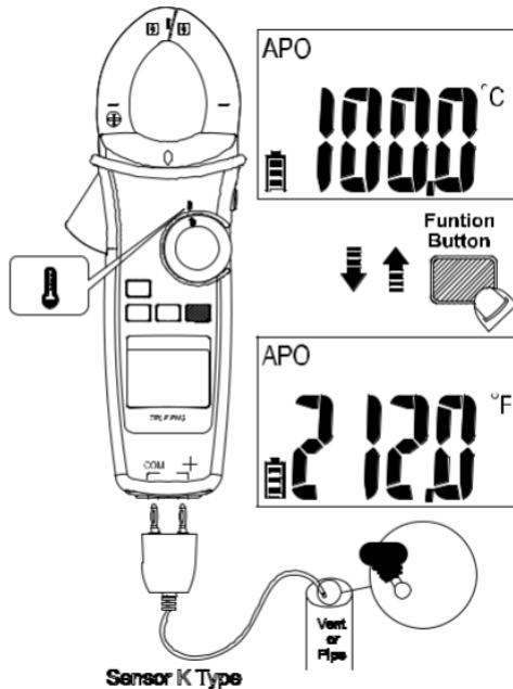
Dial the switch and press the Function button to select °C / °F mode.
