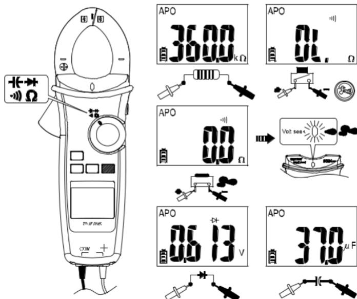
Dial the switch and press the Function button to select the measuring function.
