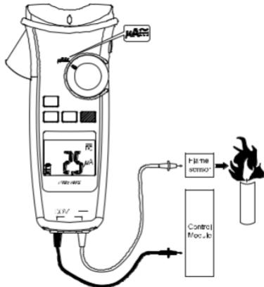
Dial the switch and press the Function button to select AC/DC mode.
