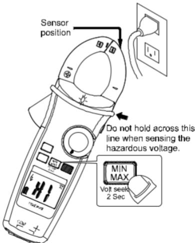
Press MIN/MAX button for over 2 sec. to enter / exit Volt Seek mode.
