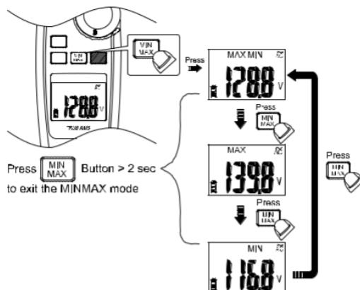
The MAX/MIN mode records the min and max input values.
