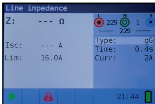
Figure 4 26: Line impedance measurement menu
