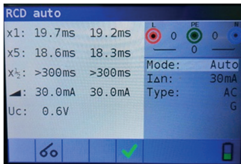
Figure 4 20: Step 8 RCD autotest results
