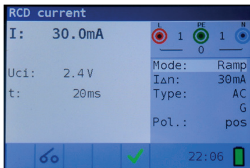
Figure 4 17: Example of trip-out current measurement result
