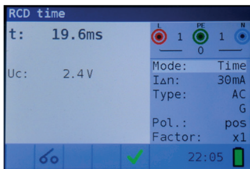
Figure 4-15: Example of trip-out time measurement results
