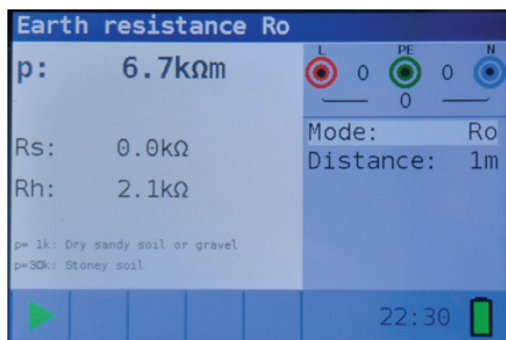
Figure 4 41: Example of specific earth resistance measurement results
