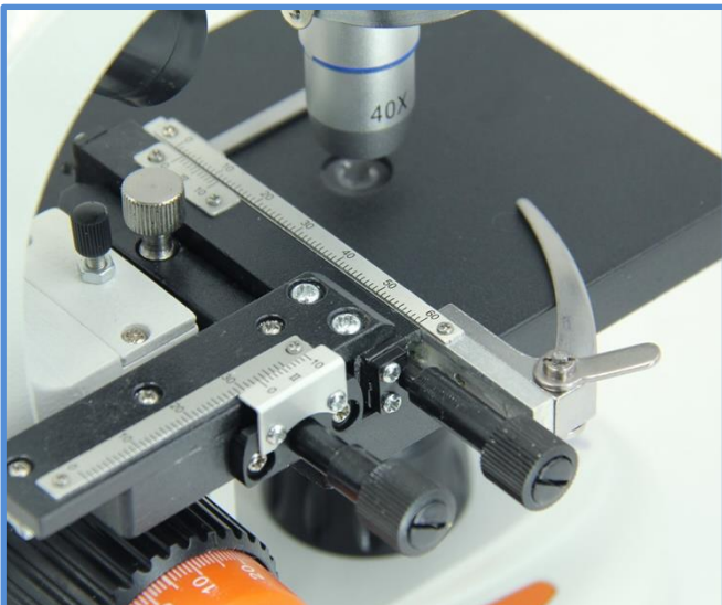
Venial scale working stage, size 95x95mm, moving range 50x30mm
