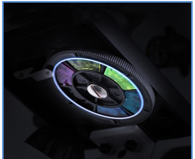
Single lens condenser, with 6 holes Disc Diaphragm and different color filters
