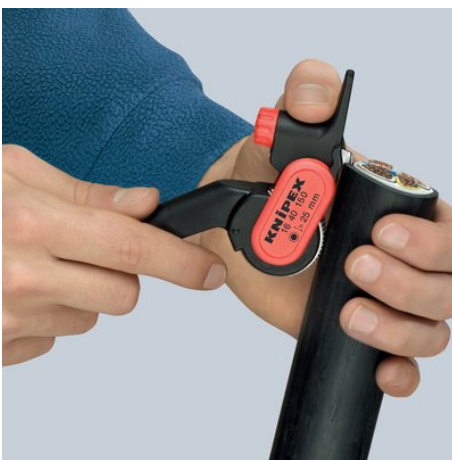
Setting the tool for longitudinal cut
