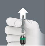
Simply push the sleeve forward to change the bit. The spring mechanism lifts the bit off the magnet and unlocks the tool. The bit can be easily removed. The rapid-out function makes it easy to remove even the smallest bits without extra tools.
