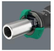
The integrated ratchet with fine toothing ensures fast and safe working. The ratchet mechanism is completely embedded in the handle. Thanks to the small size of the handle the ratchet can even be used in constricted screwdriving situations.
