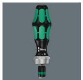
Ratchet screwdriver, fine-tooth design for minimal return angle, switchover ring (right, locked, left), maximum torque of up to 50 Newton metres, 1/4" hexagon chuck with Rapidaptor technology i.e. rapid-in, rapid-out, rapid-spin, chuck-all and single-hand function for rapid bit change, magnetic, suitable for hexagon socket insert bits as per DIN ISO 1173-C 6.3 and E 6.3 and Wera series 1 and 4
