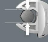
The parallel, smooth jaws of the Joker 6004 VDE offer a seating stress and can thus prevent the nut or screw head from rounding, which can occur when power is transmitted over corners.
