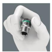
The Zyklop sockets are suitable for manual and machine-operated tools (non impact). They feature a ball stop groove and knurling at the rear end for manageability during manual use. They are made of chrome-vanadium, dull chromed. Take it easy tool finder: Colour coding by size as well as size stamping - to help you find the required socket quickly and easily.
